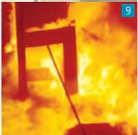
is subjected to a fully engulfing fire of 800°C for 30 minutes;
